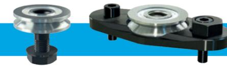
HepcoMotion Slimline Bearings are very compact due to the single ball track design. Good rigidity is maintained by a combination of ball to raceway conformity and low radial clearance, resulting in a low cost Bearing ideally suited to many Slide System applications. Performance of these Bearings has been confirmed by rigorous testing.
