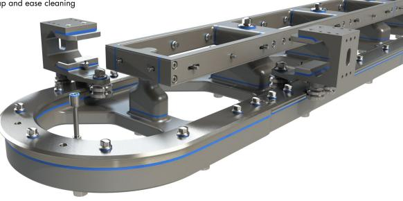
Both systems use aluminium structural components, in both the frame and the mover body. These components are hard anodized and the process reinforced with highly wear and chemical resistant additives. All slide and bearing components are martensitic stainless steel, offering good corrosion resistance and hardness suitable for bearing surfaces and consequent long service life.
