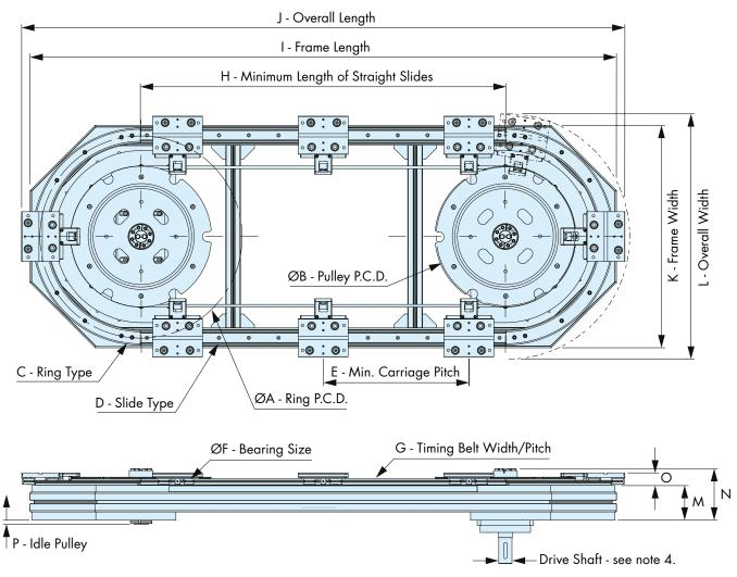
A system with 180° ring segments in an oval circuit is shown above. Rectangular systems with 90° segments are also available.
