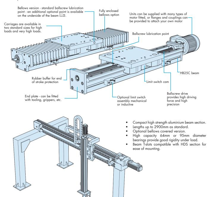
This unit uses an HDLS unit (see separate catalogue) for the X-axis and an HDCS unit with fitted servo motor for the Z-axis. A gripper is attached to the end plate of the HDCS unit.
