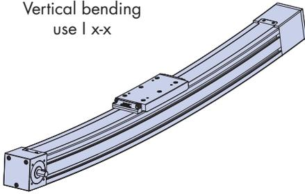
Where: E is the Young's Modulus of the aluminium material of the beam (=68,000N/mm<sup>2</sup>); I is the moment of inertia of the beam section, which can be found in the table below. The figure quoted for Ix-x is to be used when calculating deflections of beams subject to vertical bending and Iy-y is to be used when calculating deflections of beams subject to horizontal bending – see diagrams to the left and right.
