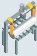
Centering mechanism with right and left thread spindles
