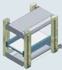
The lower and upper part of the linear freeze-dryer system is opened electro-mechanically with screw jacks for cleaning
