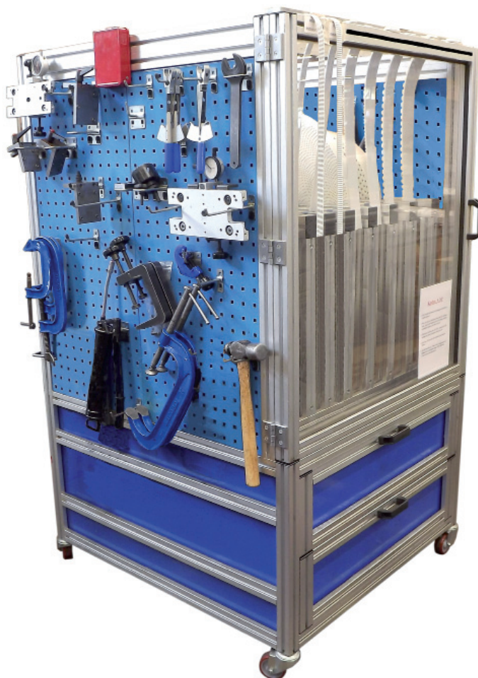
Trolley frame designed to hold a variety of equipment neatly in one place, whether on the tool rack or in one of the drawers.
