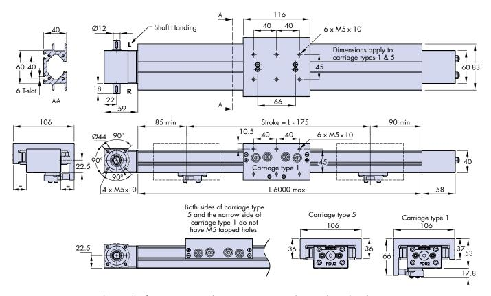
The weight of a PDU2M unit in  $kg = 1.9 + 3.36 \times L$  (where L = beam length in m).
