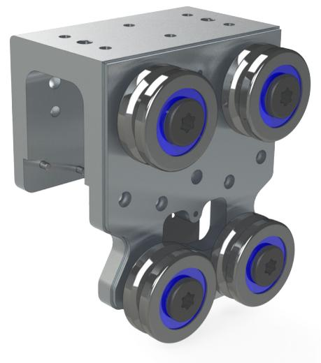
Hepco's Ø34 4 bearing PRT2 movers are available in 7 and 10 pole versions. There is also a new 4 bearing mover using the higher capacity Ø40 bearing designed specifically for the 10 pole magnet although this can be fitted with a 7 pole magnet if desired for other performance requirements.
