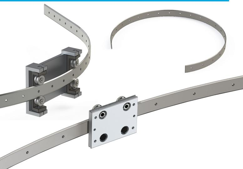
HepcoMotion Rolled Rings are a cost-effective means of achieving circular guidance of unlimited maximum diameter in commercial grade applications. Hepco Flat Slides can be rolled to any diameter above 2000mm for hardened Slides or 600mm for unhardened Slides (available for special order).
