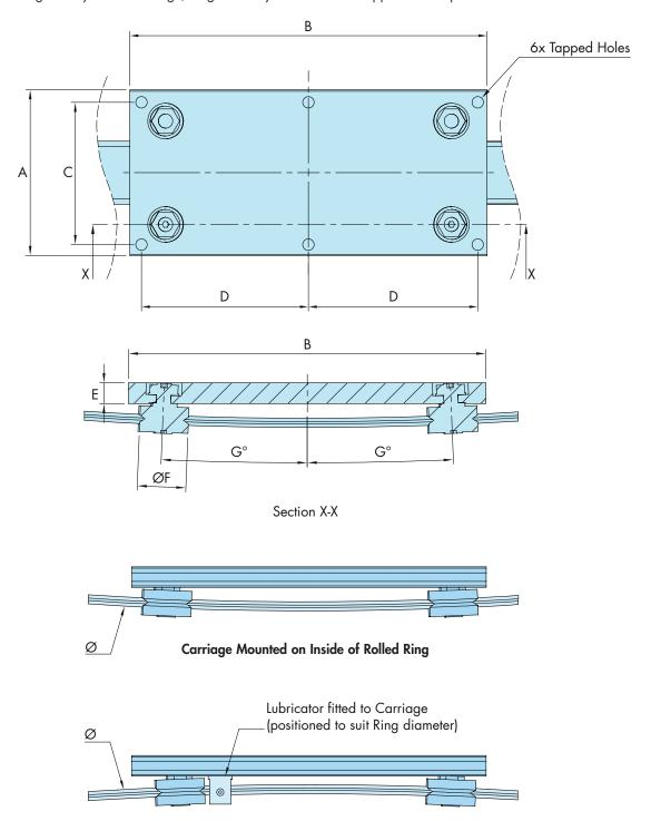
Carriage Mounted on Outside of Rolled Ring
